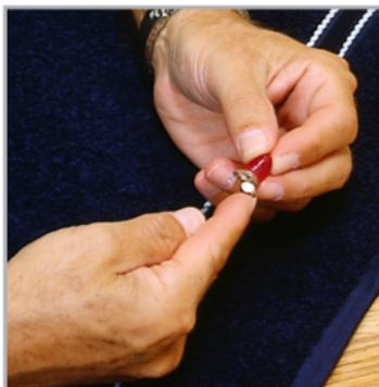
To insert or replace the battery, open the compartment by placing your fingernail under the edge of the swing-out door and gently pulling outward. **Do not open the battery door too far or damage is likely to occur.**
