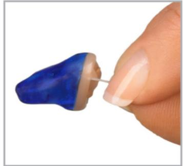
Let go of the insertion/removal line. Gently push the instrument in until it is resting comfortably inside your canal.
